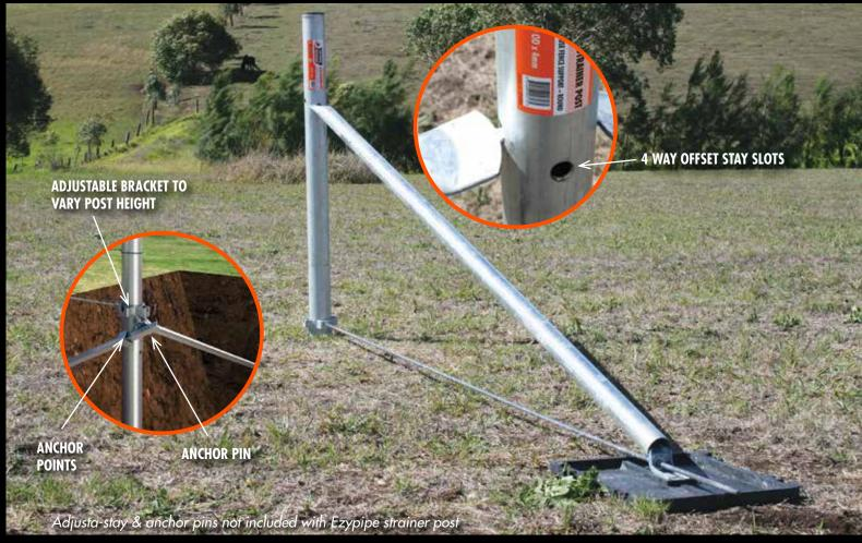
The Ezypipe strainer post is best suited to medium-soft ground applications where the greater surface area and anchor points provide improved ground holding capacity and 'jacking' resistance over other round strainer post alternatives. The Ezypipe is Waratah's round post alternative to traditional timber, pipe and concrete strainer posts that is simple to install and works with the Waratah Adjusta-stay.
